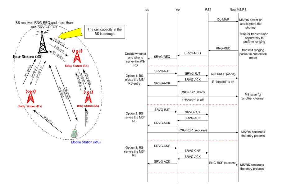
The messages sequence in MS/RS entry in multiple RS case.
