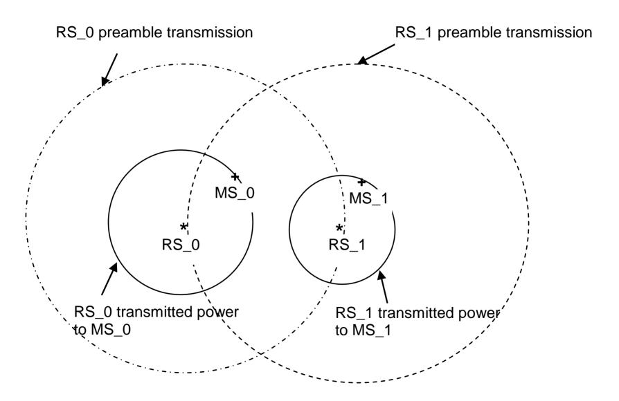
MS\_0 and MS\_1 can have channel reuse without interference
