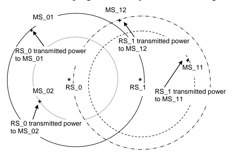
The 1st group of MS\_01 & MS\_11 and a 2<sup>nd</sup> group of MS\_02 & MS\_12 can have channel reuse without interference, but MS\_01 & MS\_12 would not be an accepted group for channel reuse due to interference.
