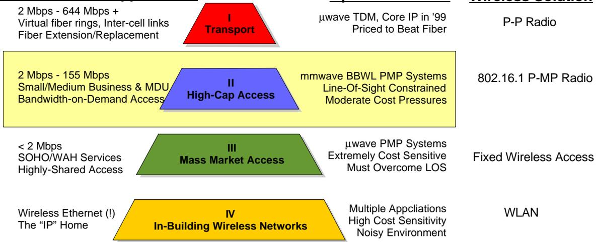
1 **Figure 1-3: A Multi-Tier Perspective of Wireless Transmission and Distribution Systems**
