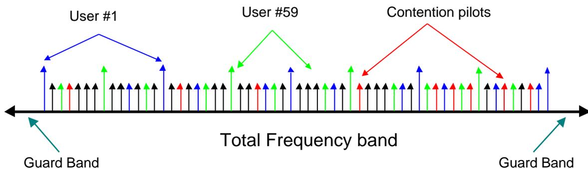
These Sub-Channels are the basic allocation unit, and the smallest granularity that a user can be allocated. Each allocation of Sub-Channel can be allocated for several OFDM symbols in such a way that the estimation of each Sub-Channels is done in frequency and time. Moreover the allocation of carriers to Sub-Channel is done by special Reed-Solomon series, which enables the optimization and dispersion of interfering signals inside a cell and between
