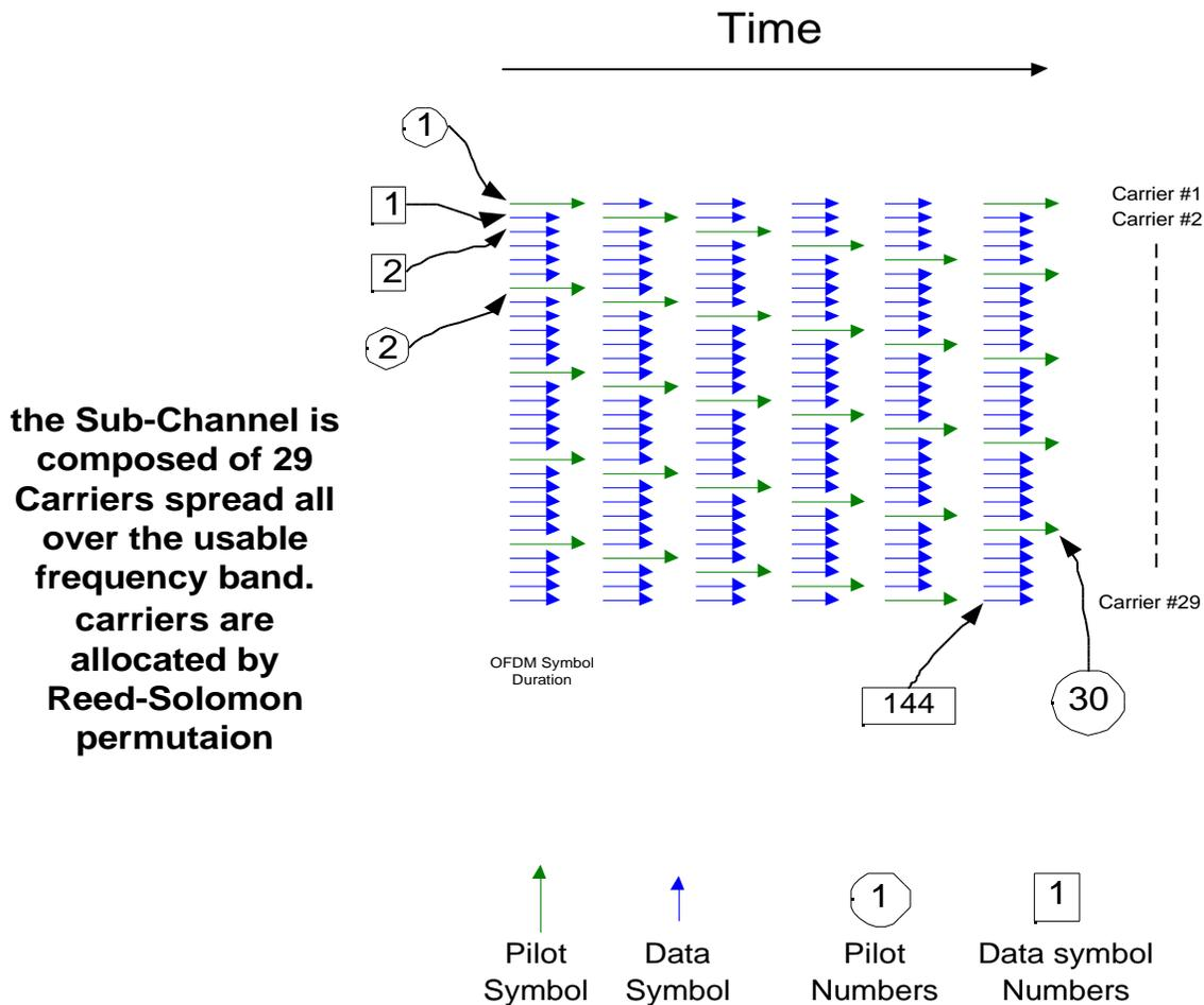
This scheme of allocation serves both frequency and time diversity. Additionally the allocation can differ to fewer carriers comprising a smaller Sub-Channel but more OFDMA symbols in time. And can be seen in the next figure:
