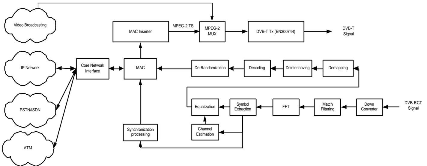
In this diagram we can see that user's Data is extracted at the Base Station and transferred by a convergence layer to the MAC. The down stream which can be composed from MAC messages or other MPEG-2 source are multiplexed into the Down Stream, the MAC messages should only be encapsulated into MPEG-2 Transport Stream, by simple means of adaptation.
