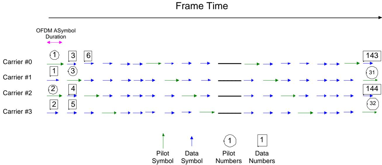
The basic 29 carriers allocation is spread all over the usable frequency range and uses special Reed-Solomon permutation to make the Sub-Channels independent as possible from each other (allocation of 4 carriers, for the mode of 4 carriers, are sub-sets of the basic Sub-Channels).
