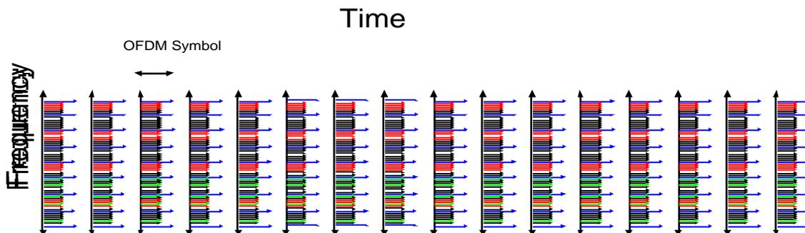
Each color in the frequency domain represents a Sub-Channel. One allocation includes allocating at least one Sub-Channel for duration of 6 OFDM symbols, this compromise is the best solution between tackling burst noise and
