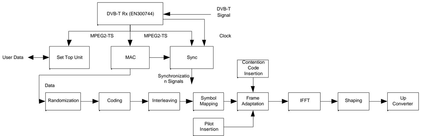
In this diagram we can notice that the user includes a simplified DVB-T receiver for the reception of the down stream. From the down stream transmission parameters and clocks are extracted and used for the upstream creation.
