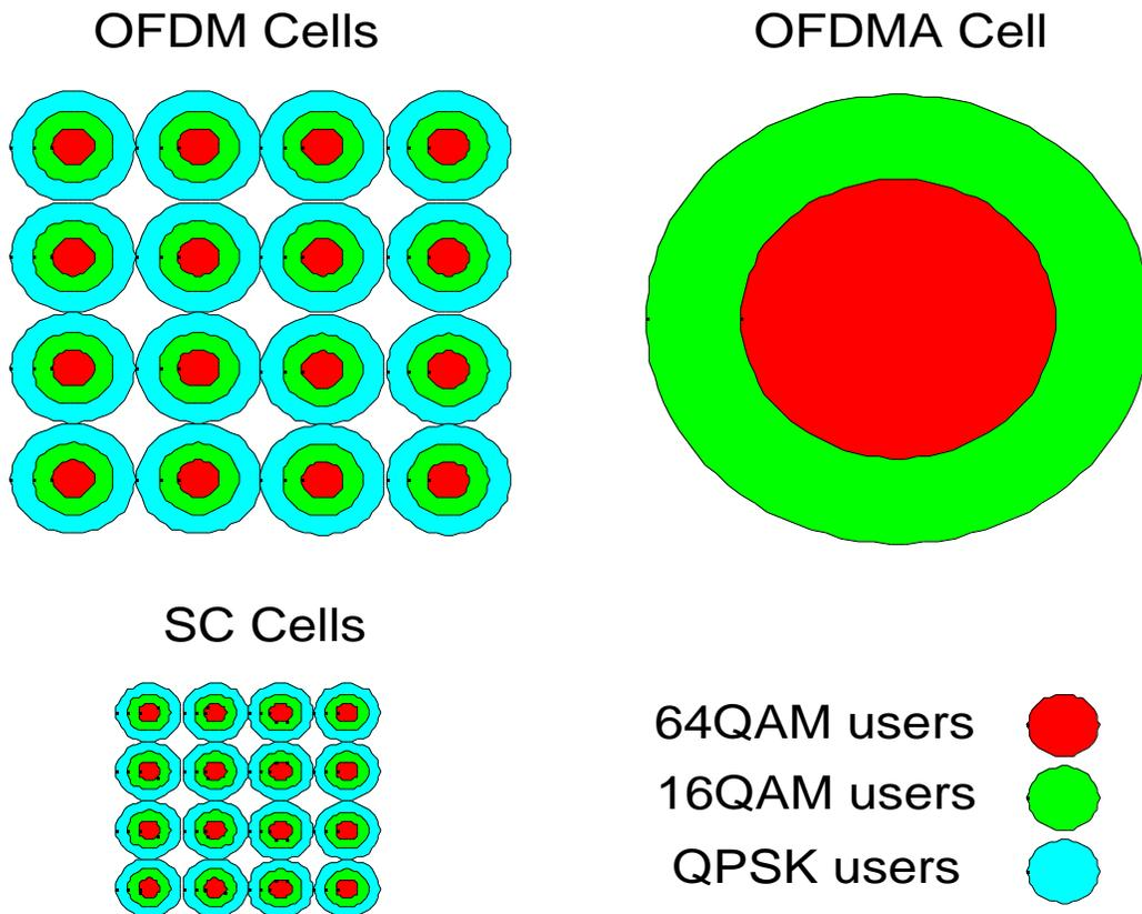
The second figure deals with the capacity issue of cells where capacity limitations are the main problem and the OFDMA system performs better due to the use of higher constellations.
