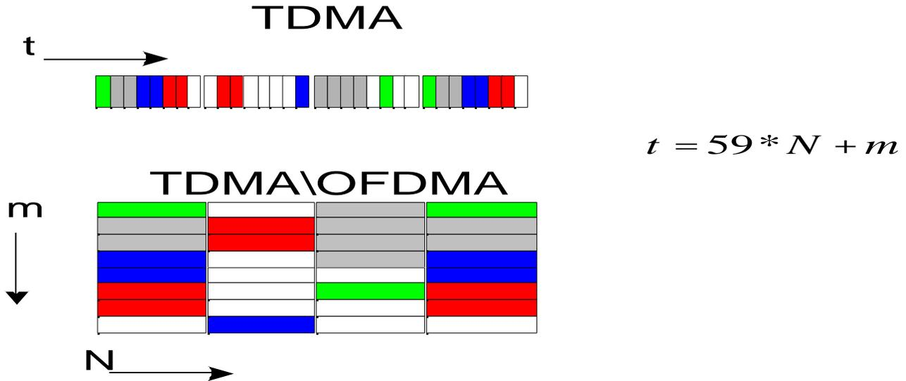
The given configuration will achieve slot granularity of ~18 bytes in QPSK with 1/2 code rate.
