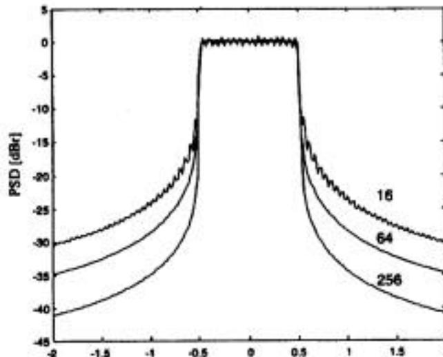
The figure illustrates the decay of the OFDM symbol when using different sizes of FFT as we can see 6dB reduction is achieved by quadrating the number of points therefore the difference between 64 points and 2048 points is about 15dB. The figure shown above is for rectangular windowing, the signal can be further perfected by adding windowing at the start and at the end of the signal, by that a DVB-T modulator can reach an 85dB decay 1/20 the frequency band away, as seen in the next figure:
