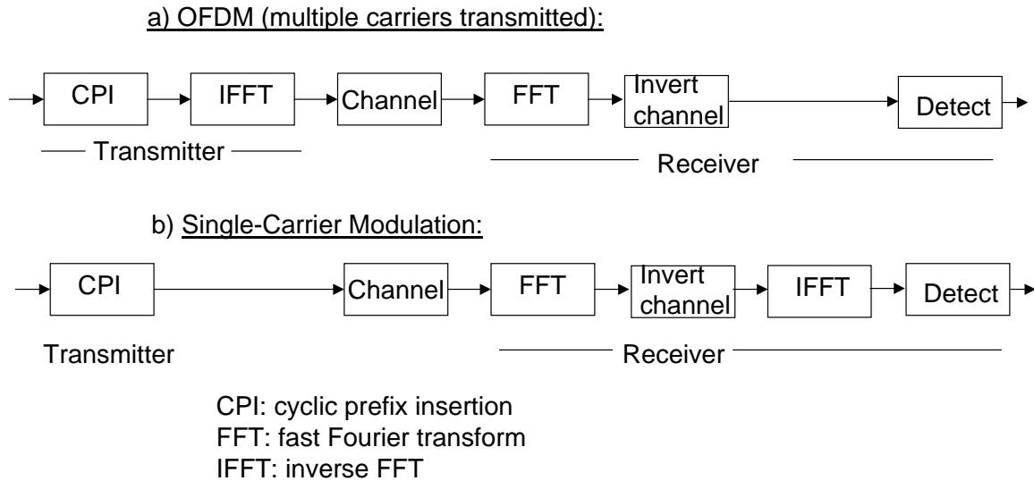
**Figure 11- OFDM and Single Carrier-Frequency Domain Equalization (SC-FDE).**
