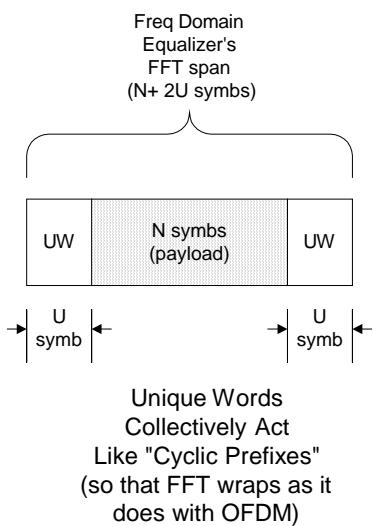
**Figure16: Structure of equalizer which can be exploited by frequency domain equalization.**
