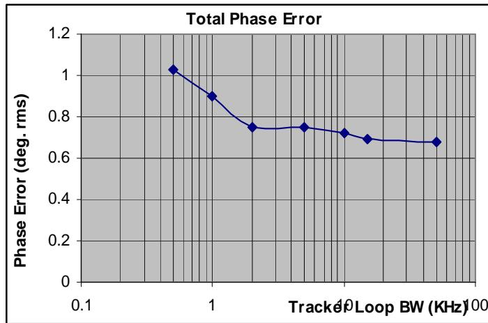
**Figure 17: Total RMS Receiver Phase Error**
