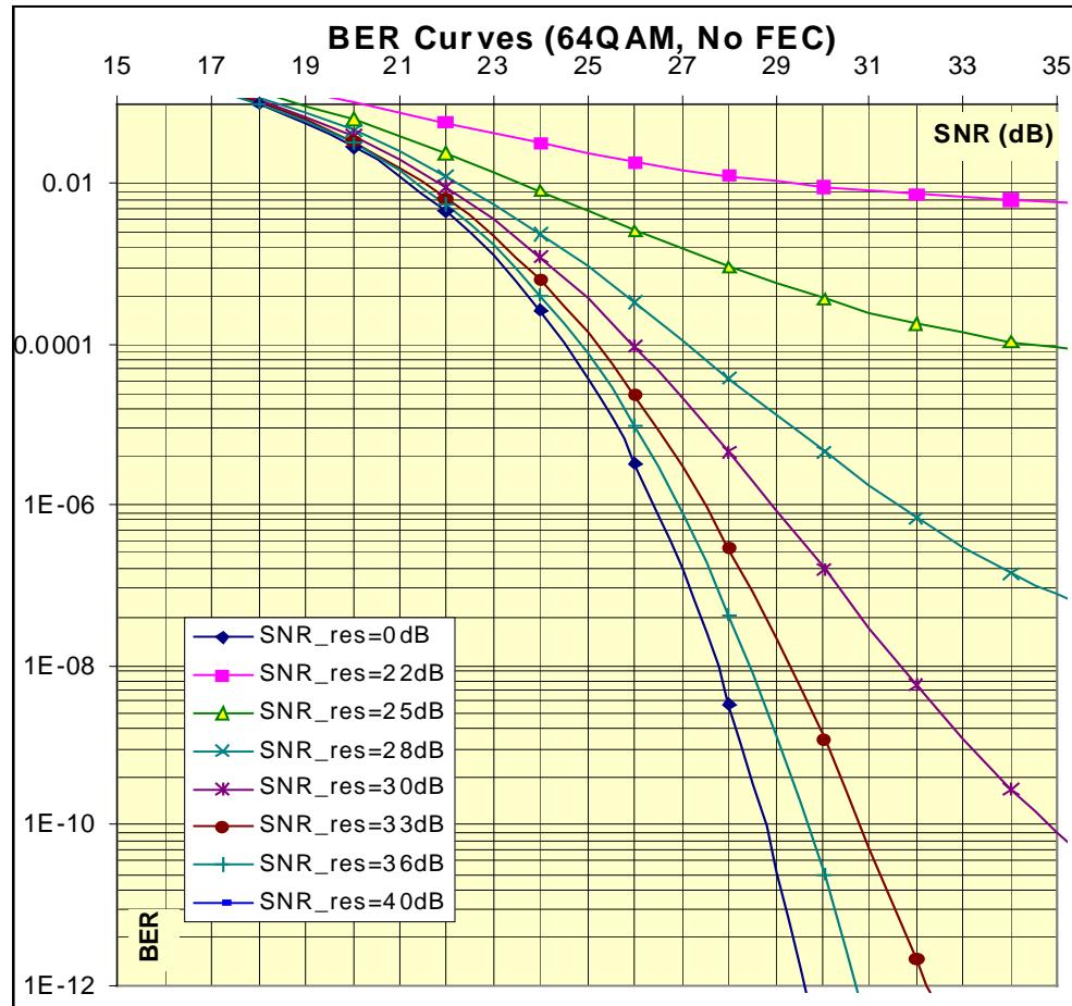
**Figure 18: BER vs SNR for various residual SNR**
