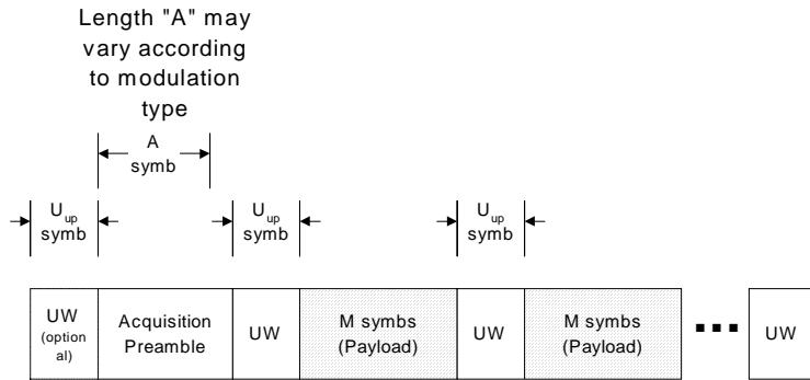
**Figure 15: Framing Structure for Upstream (for simplicity, gaps due to potential downstream TDD framing structure omitted).**
