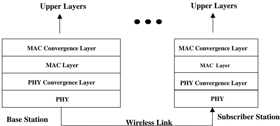
**Figure 3: The proposed PHY Layer with upper layers protocol stack.**
