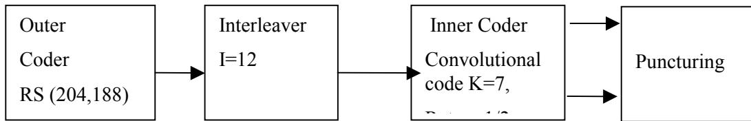
**Figure C5 – Concatenated Reed – Solomon and Convolutional Codes Encoder Block.**
