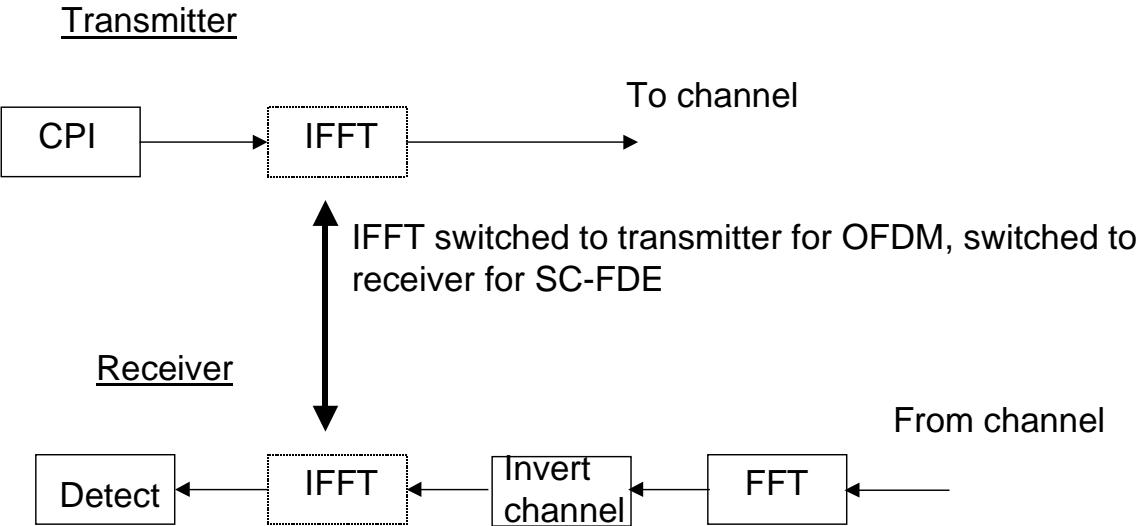
Figure 12 - OFDM and SC-FDE “Convertible” Modem Approach.
