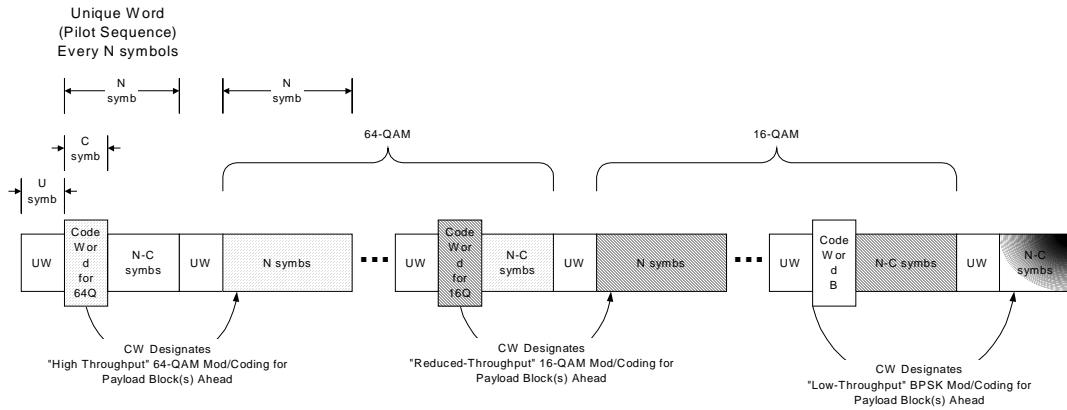
**Figure 13: Framing Structure for FDD system; Downstream.**
