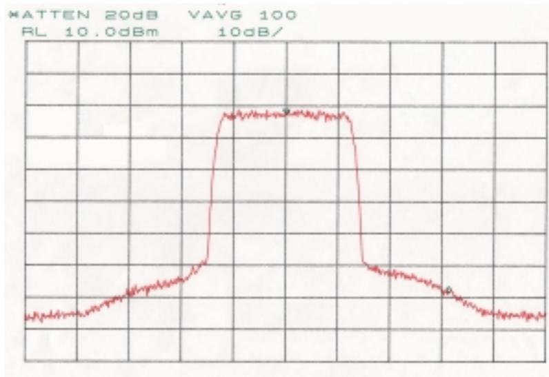
Figure 20: 64 QAM at 9 dB back off
