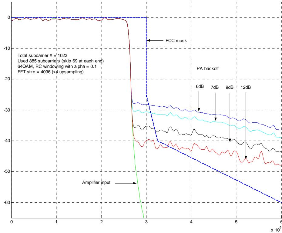
**Figure 21: OFDM at various back-off levels**
