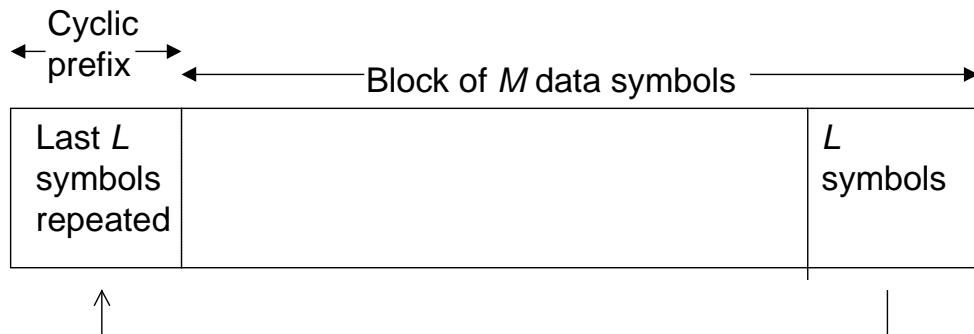
Figure 13 - Block Processing in Frequency Domain Equalization
