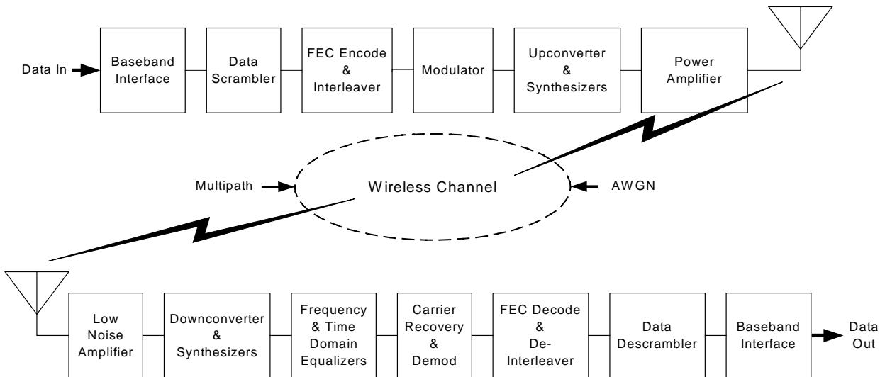
**Figure 2: The Proposed Single Carrier PHY Layer Block Diagram.**
