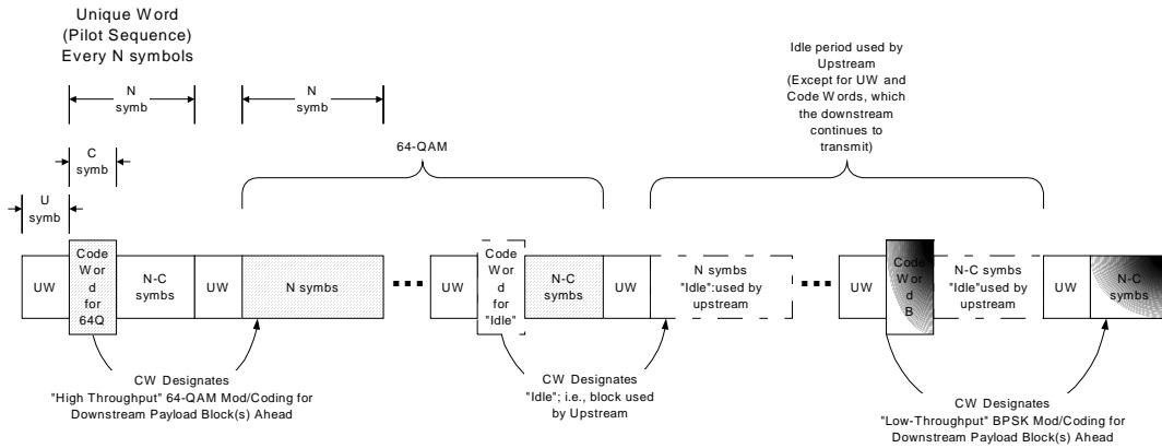
**Figure 14: Framing Structure for TDD system; Downstream.**
