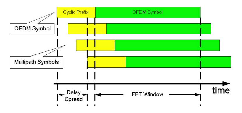
Inter-symbol interference is further reduced by incorporating a cyclic extension to each OFDM symbol.
