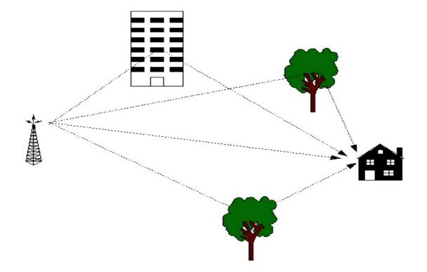
• Frequency selective fading is caused by reflectors between the transmitter and receiver creating multipath effects.
