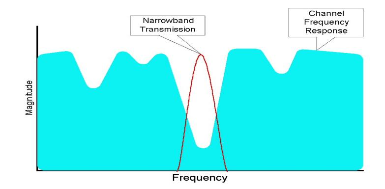
• For narrow bandwidth transmissions, if the null in the frequency response occurs at the transmission frequency then the entire signal can be lost.
