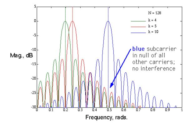
The inverse DFT ensures that the spacing and the spectral shape of the sub carriers are such that the spectra of the individual sub carriers is zero at the other sub carriers. That is, the sub channels are orthogonal.
