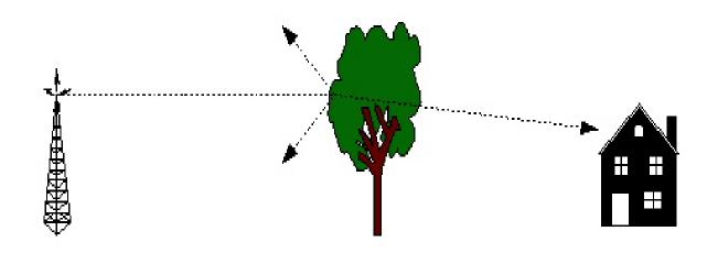
• Flat fading is caused by absorbers between the two antennae and is countered by antenna placement and transmit power level.
