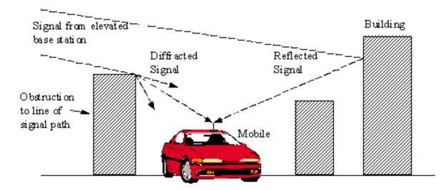
As well as creating frequency select fading, multipath can also cause inter-symbol interference.
