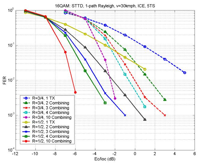
• FER versus Ec/Ioc for 16QAM. STTD on, 1-path Rayleigh channel, speed = 30Kmph, ideal channel estimation, frame length=3.33ms, HARQ with Chase Combining
