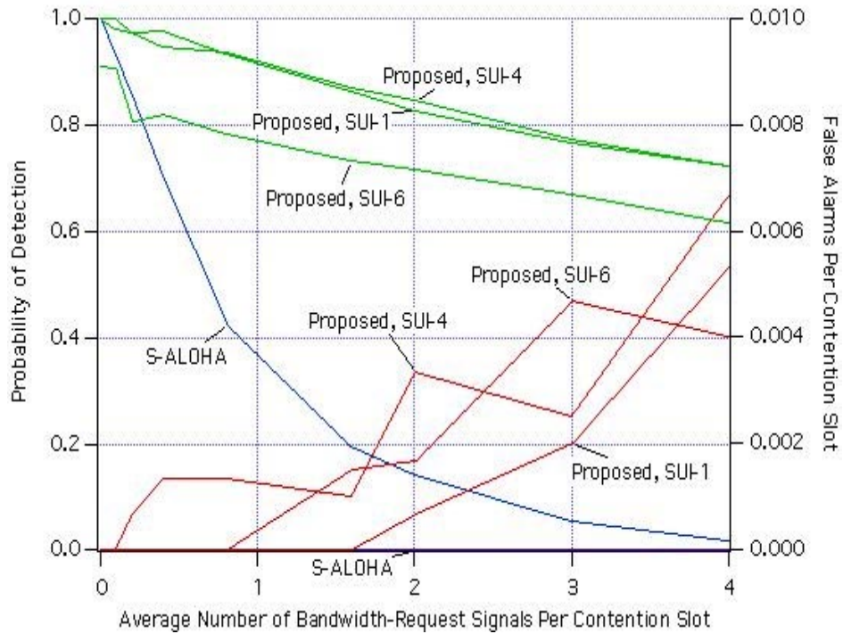
Figure 4. Performance, Proposed System with 16-bit codes, 99 dB SNR, no retransmits.
