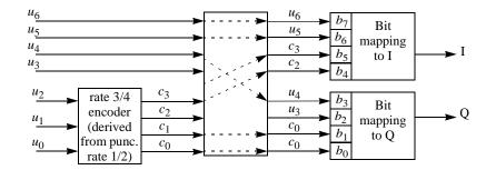
Figure 162—Optional pragmatic TCM encoder for rate 7/8 256-QAM
