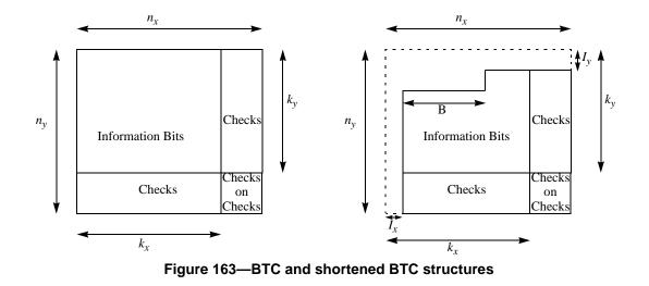
An extended Hamming component code shall use n-k check bits. The first n-k-1 check bits are the check bits of a (n-1, k) Hamming code derived from one of the generator polynomials listed in Table 156, while the last check bit is a parity check bit, derived by XORing the n-1 information and parity bits of the (n-1, k) Hamming code.
