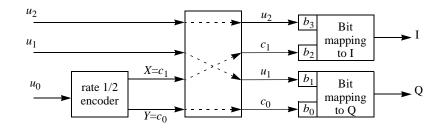
Figure 158—Pragmatic TCM encoder for rate 3/4 16-QAM
