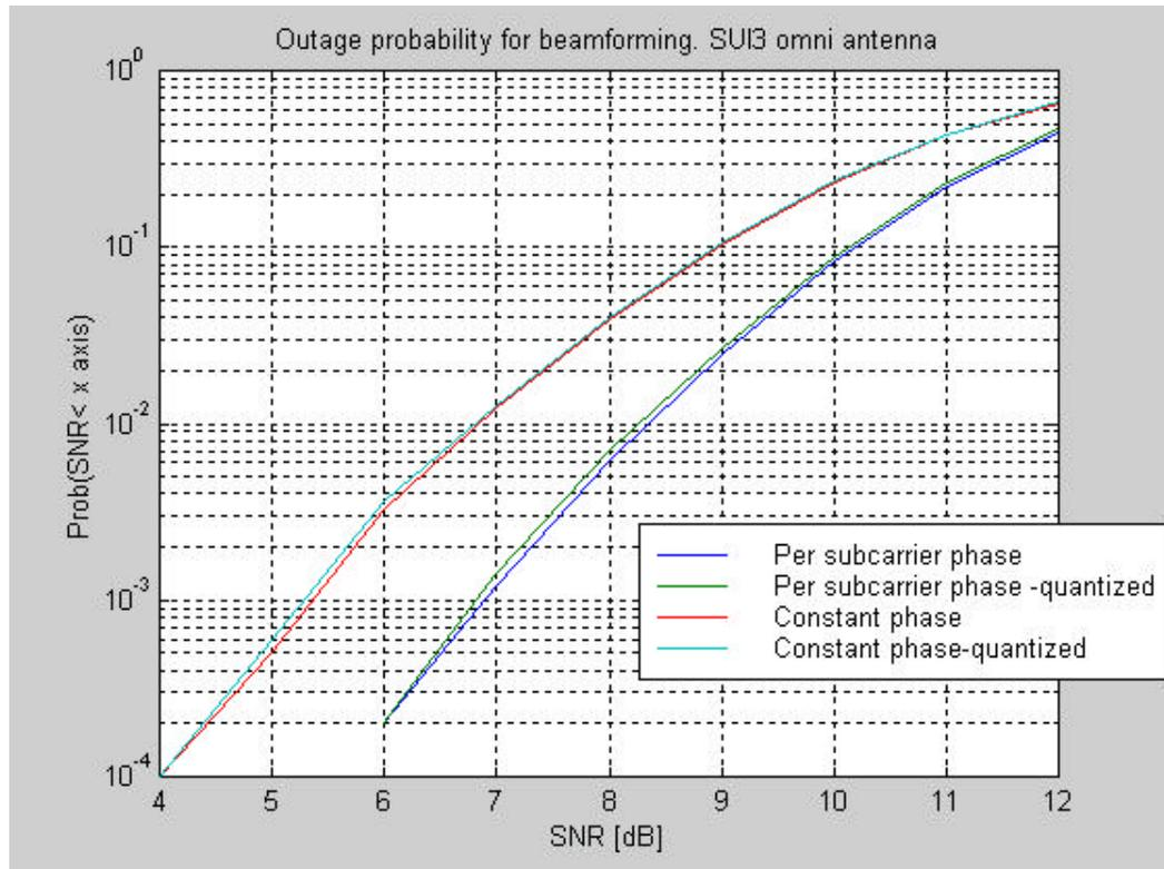
As can be seen for the difference between per-subcarrier and constant phase, @Poutage= $10^{-3}$  are about 1.5dB.
