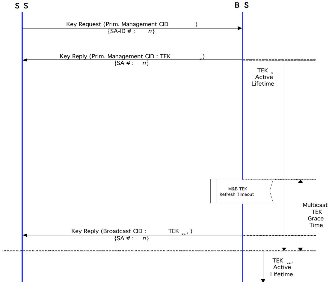
**Figure 0.1 TEK management for the multicast and broadcast service**
