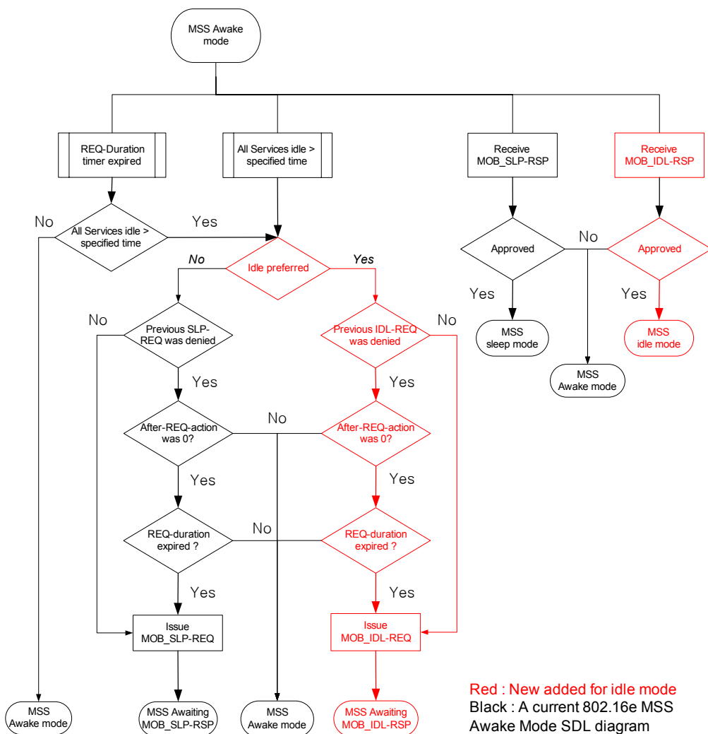
Figure. 108a - MSS Awake Mode SDL Diagram
