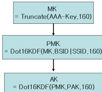
Figure 4. AK derivation mechanism in PKMv2
