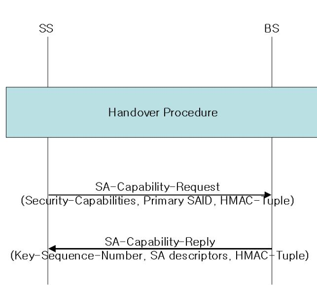
Figure 6. the flow when the pre-authentication is used
