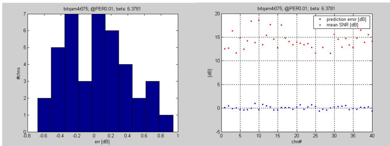
Figure 5 - 16-QAM  $\frac{3}{4}$ : (left) EESM fit error, (right) mean SINR and prediction error per channel realization
