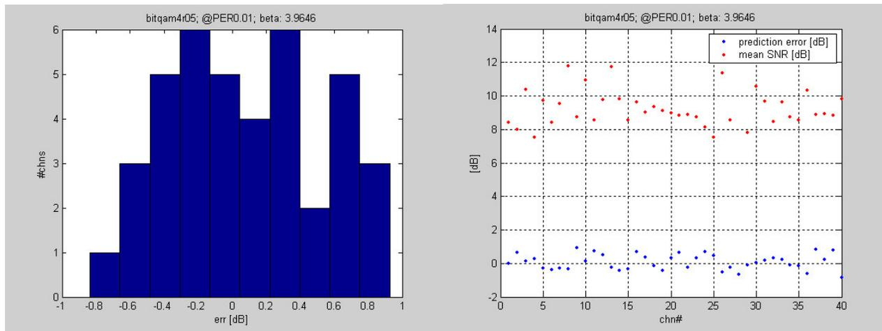
Figure 4 - 16-QAM  $\frac{1}{2}$ : (left) EESM fit error, (right) mean SINR and prediction error per channel realization
