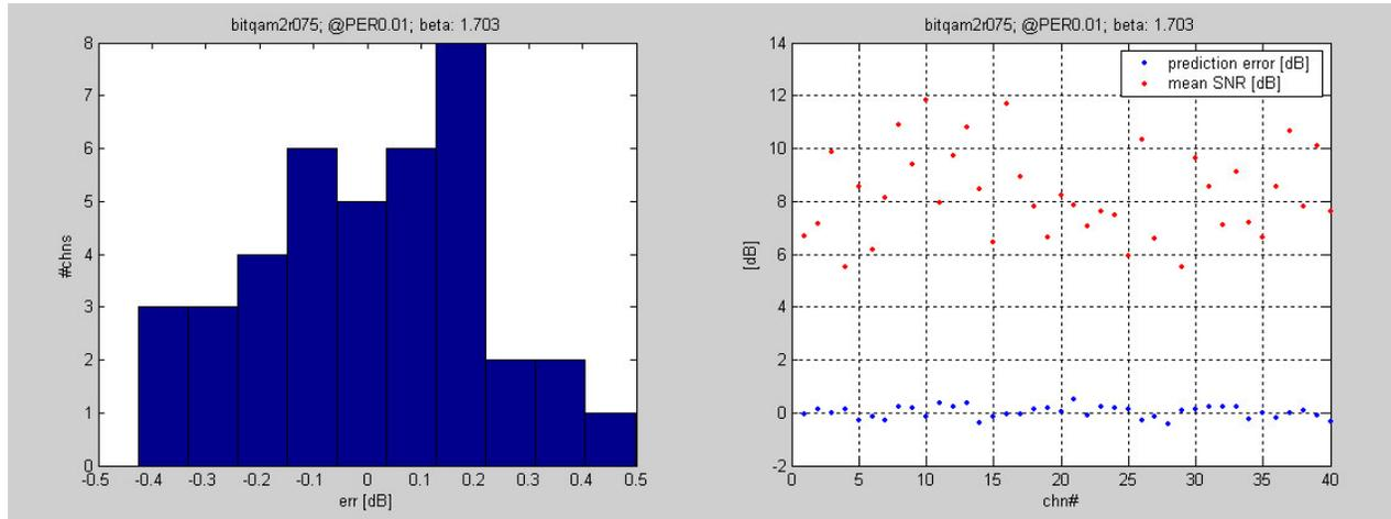
Figure 3 - QPSK  $\frac{3}{4}$ : (left) EESM fit error, (right) mean SINR and prediction error per channel realization
