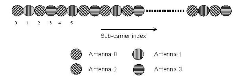
Figure xxxx. Midamble FUSC structure (frequency domain)
