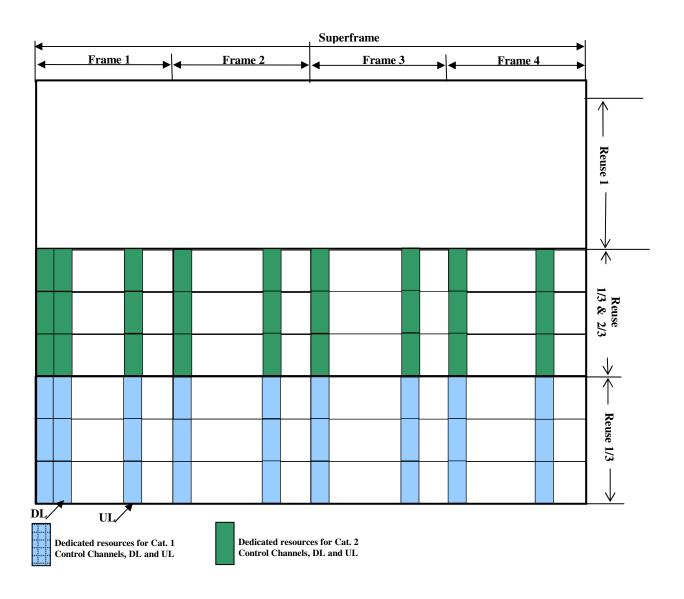
Fig. xx Control channels allocations for Relays and Macro BS
