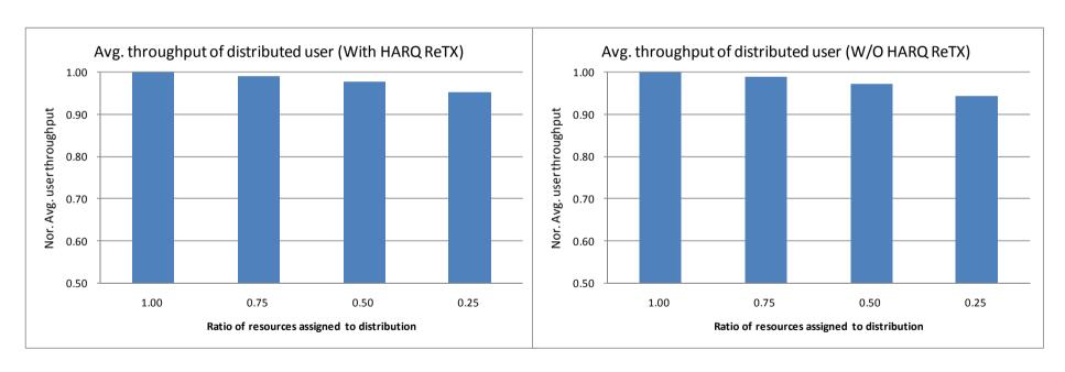
Diversity loss due to FDM MUX is about 2~3% when half of resources are used for diversity.
