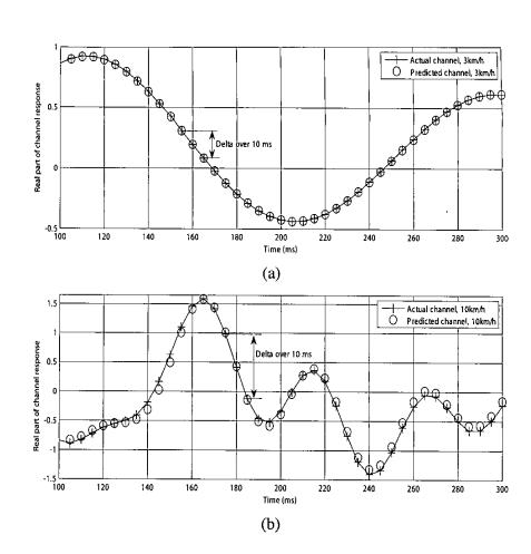
Fig. 2. Time varying fading channels and the predicted channel responses for mobile speeds: (a) 3 km/h, (b) 10 km/h.
