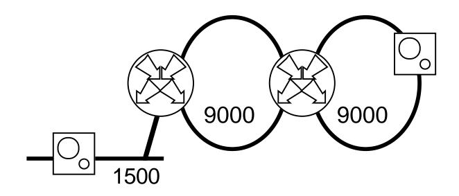
RPR->Ether->RPR, routed Handled: Path MTU Discovery
