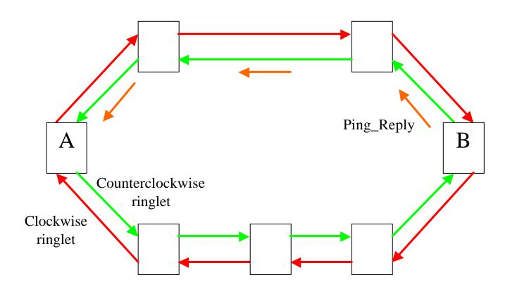
When node B receives the RPR Ping Request, it generates the RPR Ping Reply to node A
