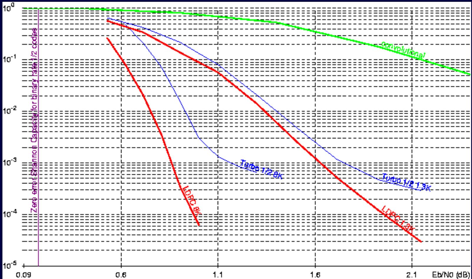
Comparison of LDPC codes, Turbo codes and IS-95 convolutional code of rate 1/2
