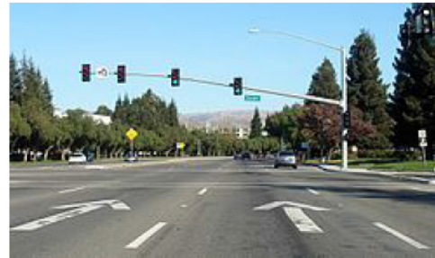
Thru lanes indicated by arrows on California CR G4 (Montague Expressway) in Silicon Valley.
