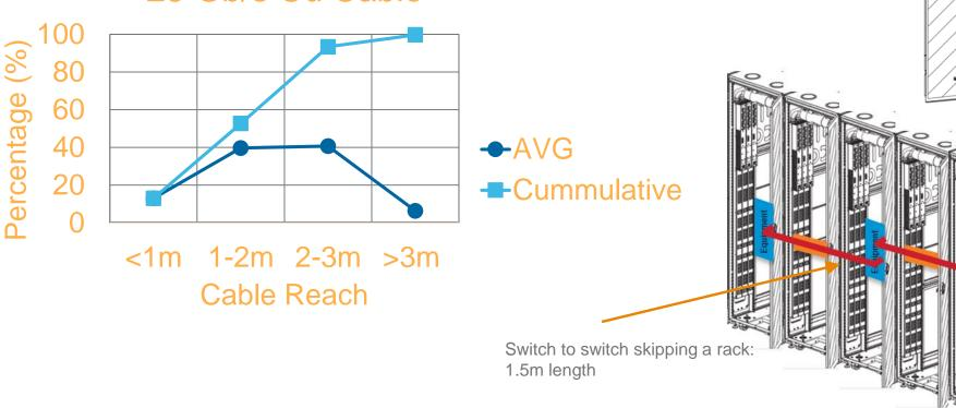
Data center architectures can be configured for <2m length to enable usage of low cost copper cables
