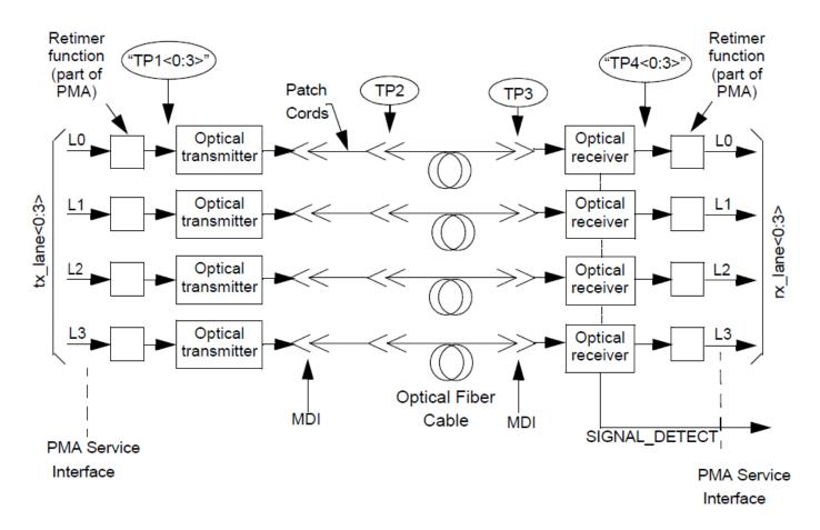
TP1 and TP4, shown here for illustration only, represent the start and end of link budget calculations. They are not accessible points for measurements, nor intended as reference points for specifications
