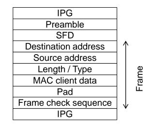
The first octet of the preamble is mapped to a start control character by the RS and is always aligned to the start of a 64-bit block. Consequently, a 64 octet frame will be encoded as a Start 64-bit block (which contains the Preamble and SFD), followed by eight 64-bit blocks containing the MAC frame, followed by a Terminate 64-bit block containing 7 Idle control characters – 10 64-bit blocks in all with minimum interpacket gap.
