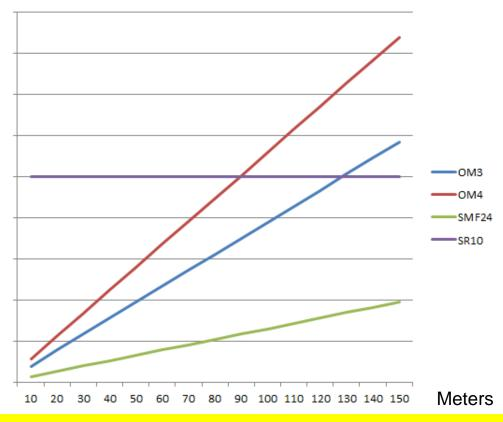
24-Fiber SMF cable is half the cost of 12 duplex SMF cables, 1/3 the cost of 24f OM3 and 1/4 the cost of 24f OM4
