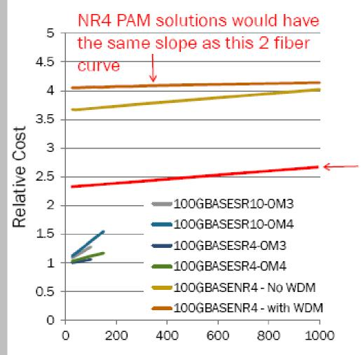
NR4 no WDM (8 fibers) is assumed to be 20% less cost than NR4 with WDM (2 fibers). The NR4 no WDM is less cost up to 1000m.
