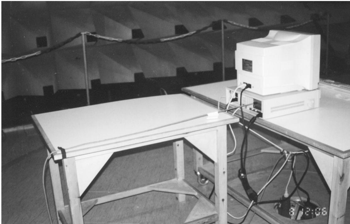
Fig 6 Radiated emission set-up according to CISPR 22.
