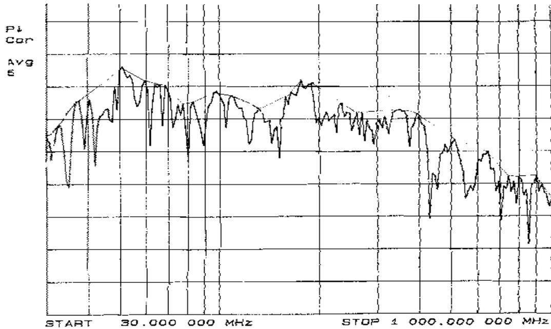
Fig. 4. Site attenuation of cabling set-up. Common mode excitation.
