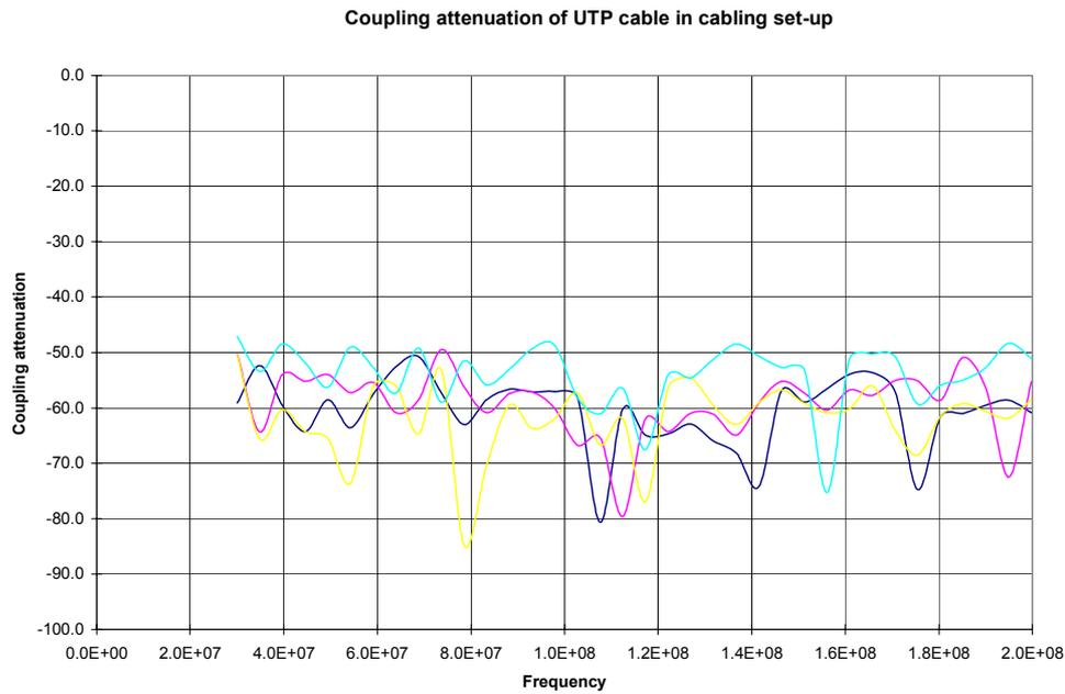
Fig. 19. Coupling attenuation for UTP cable.
