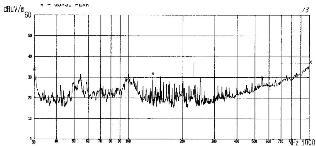
Fig. 10. Radiated emission. PC connected to UTP link.
