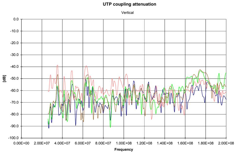
Fig. 17. Coupling attenuation for UTP link
