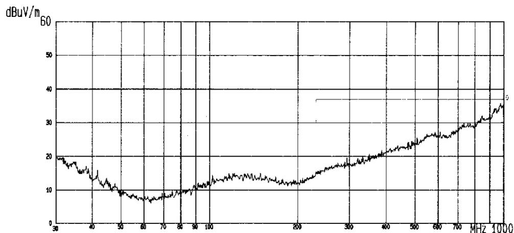
Fig. 13. Emissions from S-FTP cabling. Active equipment outside test chamber.
