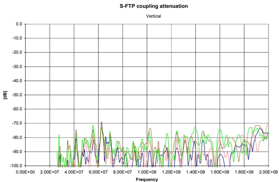
Fig 18. Coupling attenuation for S-FTP link
