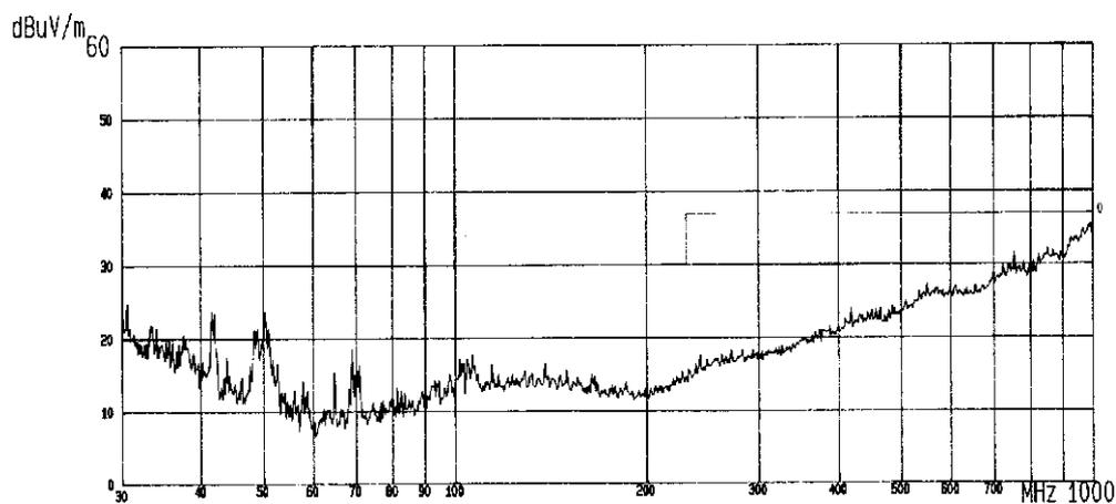
Fig. 12. Emissions from UTP cabling. Active equipment outside test chamber.
