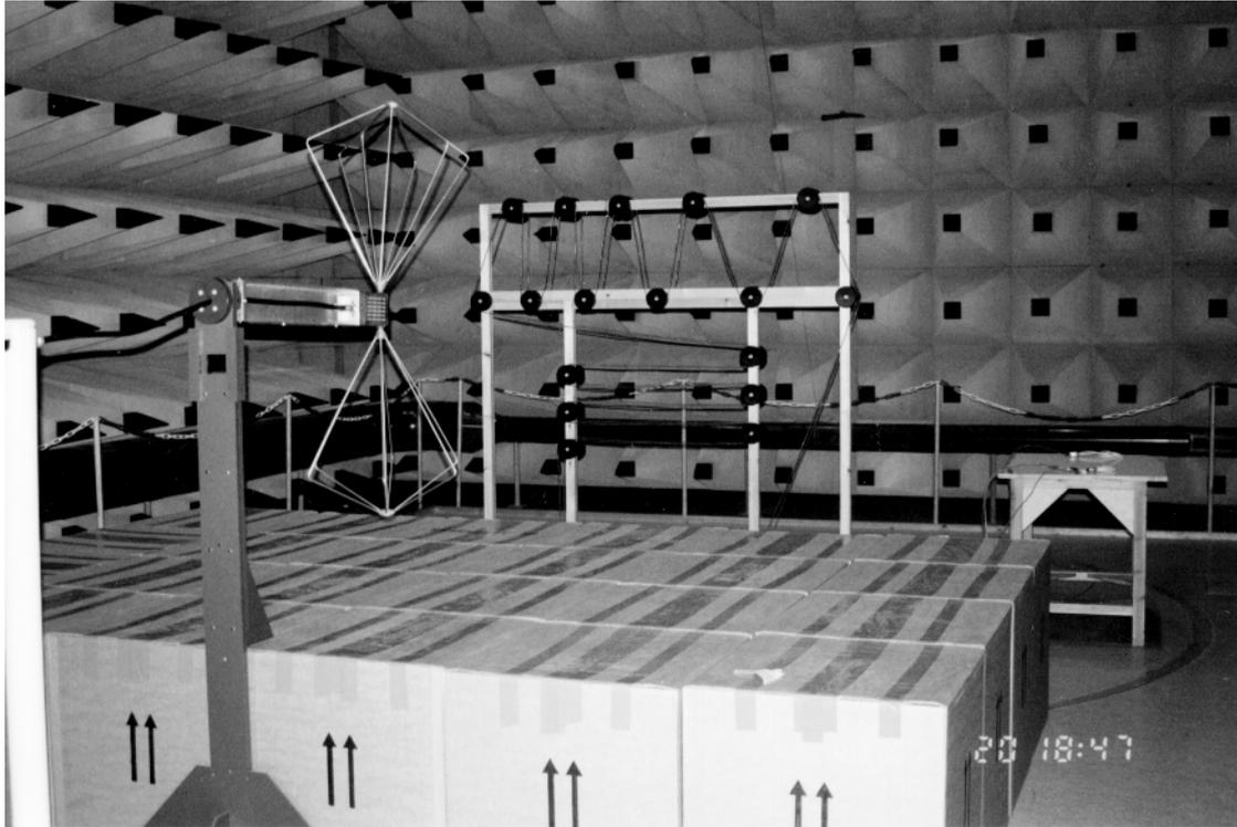
Fig. 14. Test set-up for immunity measurements.
