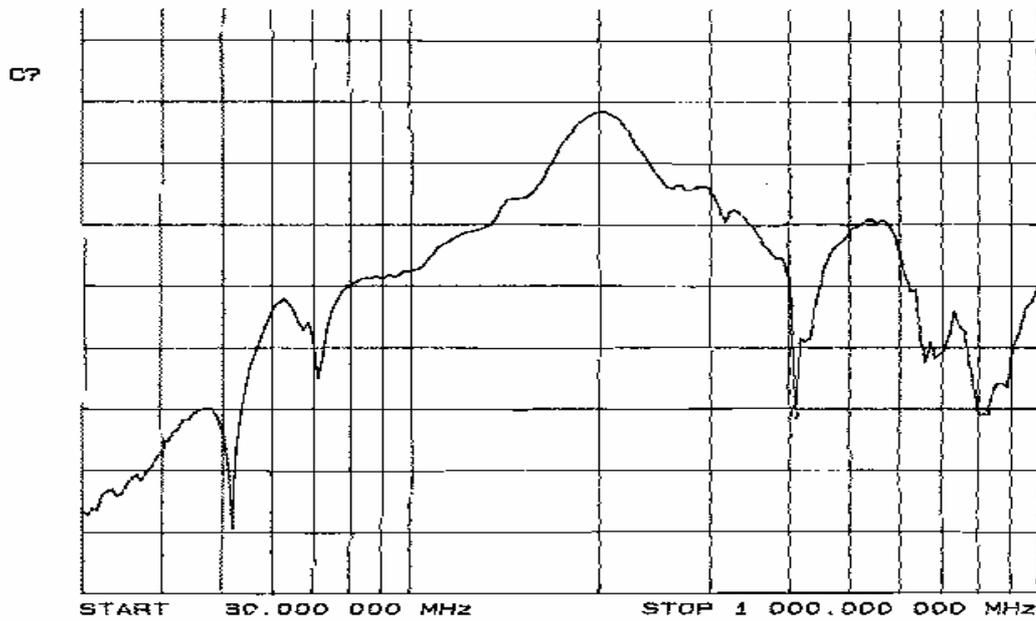
Fig. 5. Site attenuation of dipole adjusted for resonance at 200 MHz.
