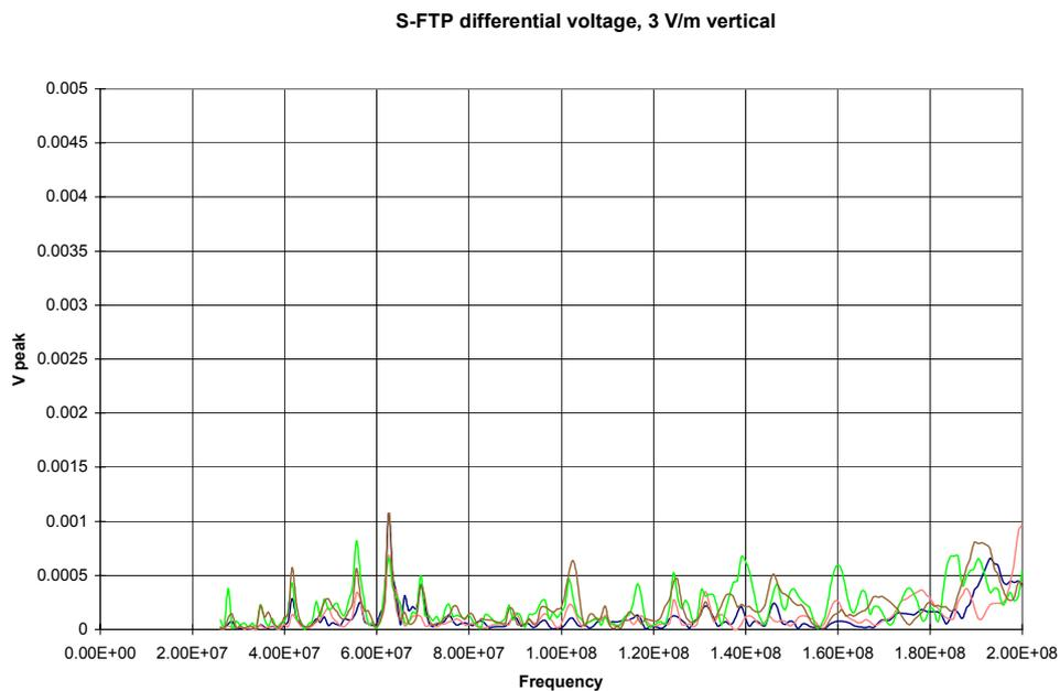
Fig. 16. Voltage at cabling interface, S-FTP cabling (vertical polarisation)
