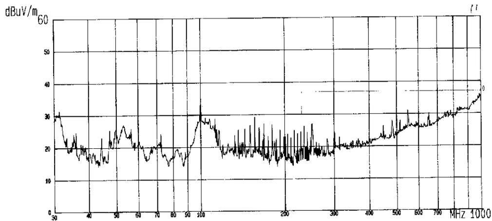
Fig. 11. Radiated emission. PC connected to S-FTP link.
