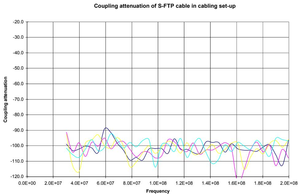
Fig. 20. Coupling attenuation for S-FTP cable.
