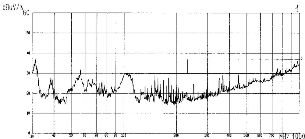
Fig. 7. Radiated emission for PC with UTP cable.
