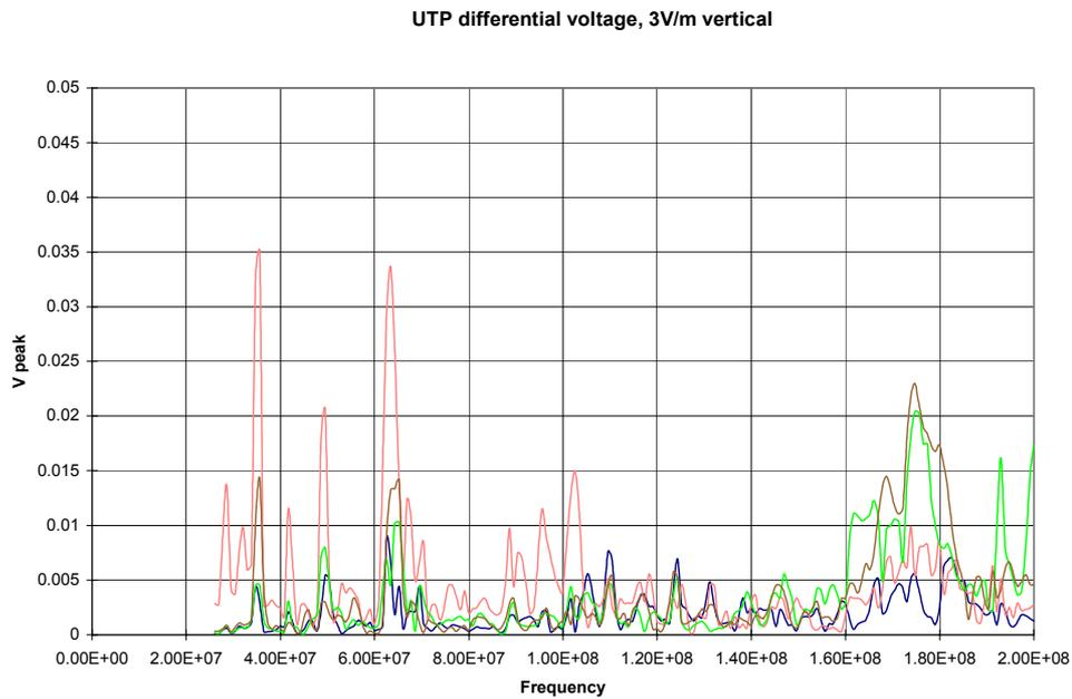
Fig. 15. Voltage at cabling interface, UTP cabling (vertical polarisation)
