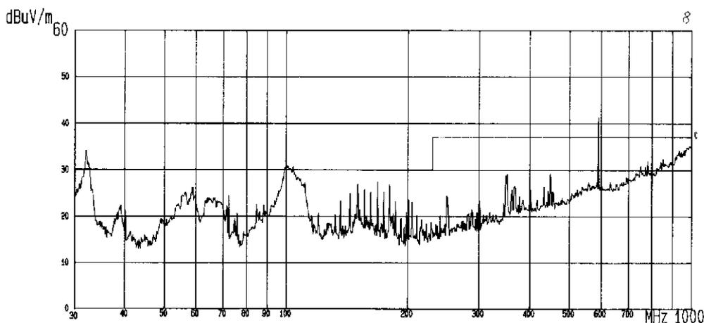
Fig. 8. Radiated emission for PC with S-FTP cable.
