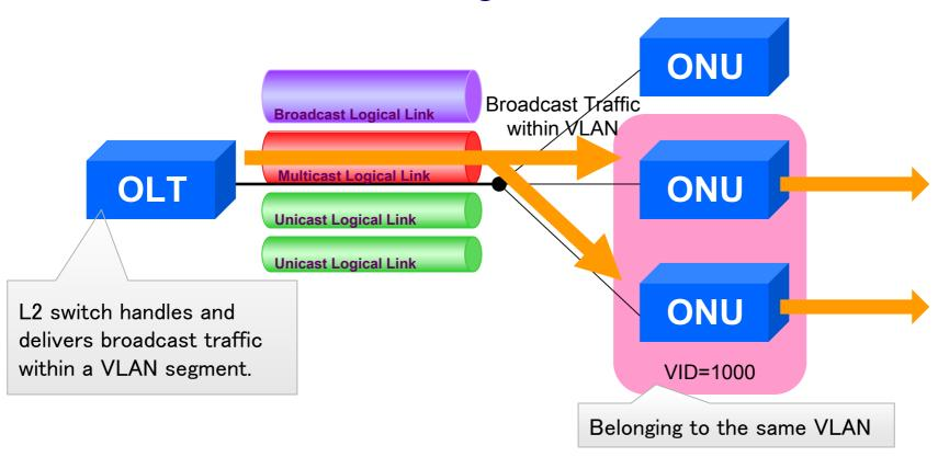
Only OLT is responsible for handling VLAN switching. ONU can be a repeater without a processor.
