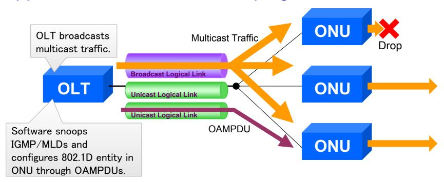
Need an 802.1D entity in ONU. Need to specify proprietary OAMPDU messages. Affect multicast performance due to OAMPDU delay time.
