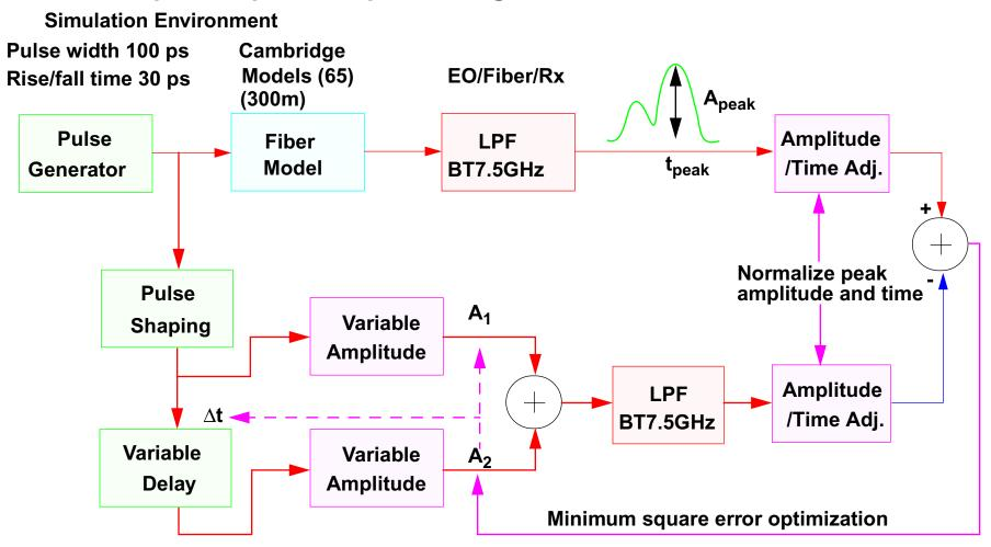
The simulation environment for fiber path consists of the fiber model (Cambridge model), a BT LPF 7.5 GHz and a normalization block to adjust for peak amplitude value and time.
