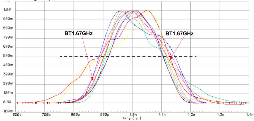
For symmetrical and non-symmetrical pulse response fibres, the maximum error at the slicing level (BT1.67GHz output amplitude 500 mV) is 150 mV (30%)
