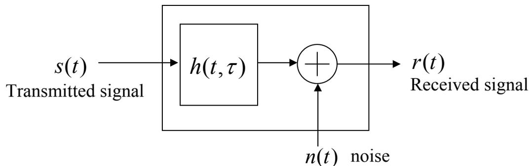
Here  $n(t)$  represents sum of all noise terms, and  $h(t, \tau)$  represents time-varying impulse response. Multimode fiber impulse response can be modeled as that of a multi-path channel.
