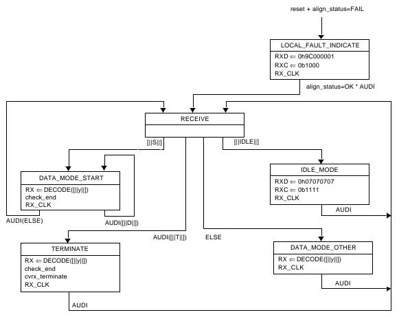
Figure 48–9—PCS receive state diagram
