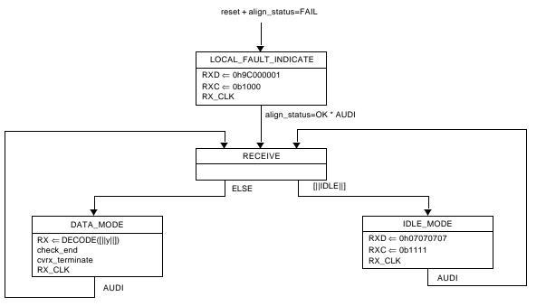
Figure 48–9—PCS receive state diagram
