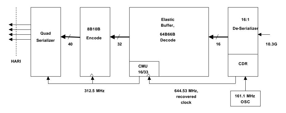
There is one clock/jitter domain in the receive path – the link clock, recovered from received serial data. The 161M OSC is used as a REFCK to Clock and Data Recovery circuit inside the de-serializer. The clock required for 8B10B encode and Quad-Serializer is derived by multiplying the link clock with 16/33.
