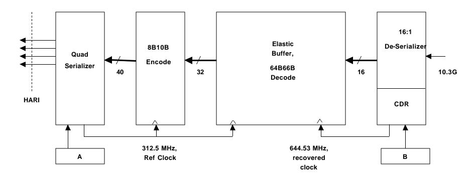
There are two clock/jitter domains in the receive path – link clock domain and HARI clock domain. Link clock is recovered from received serial data. Here B, the 644M OSC, is used as a REFCK to Clock and Data Recovery circuit inside the de-serializer. And A, the 312.5 MHz OSC, is used as a reference clock for the HARI clock domain.
