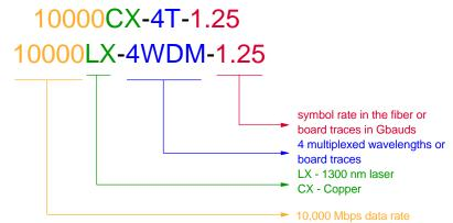
meters. The solution includes some reuse of prior 1 GE PCS technology. The CX solution is great for backplane runs at a meter or less with current standard layout techniques and PCB materials. By mixing the two technologies one can develop media converters. This technology is already running in simulation and first prototypes are expected by 1Q01.
