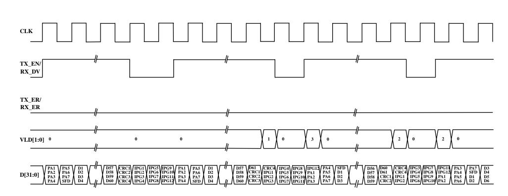
Notes: - When TX\_EN/RX\_DV is asserted, an encoding of VLD=0 indicates four valid bytes on D[31:0].
