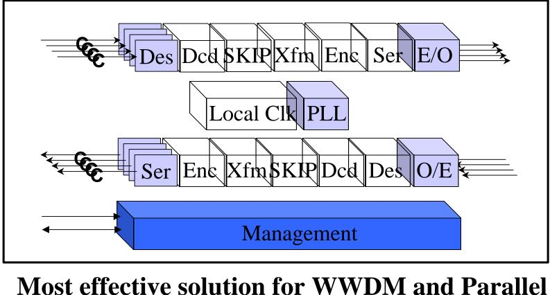
Most effective solution for WWDM and Parallel if local clock is not required and PHY can meet jitter requirements.
