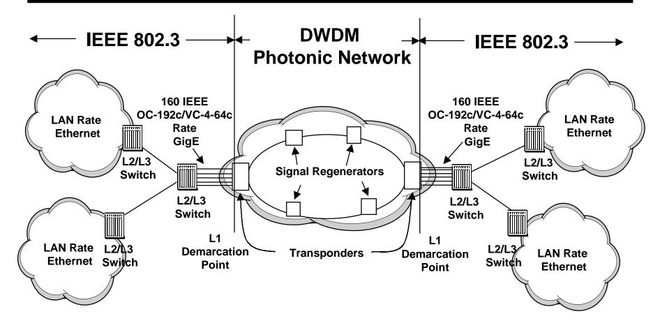
LAN Switches de-couple the LAN Rate and WAN Rate PHYs by buffering
