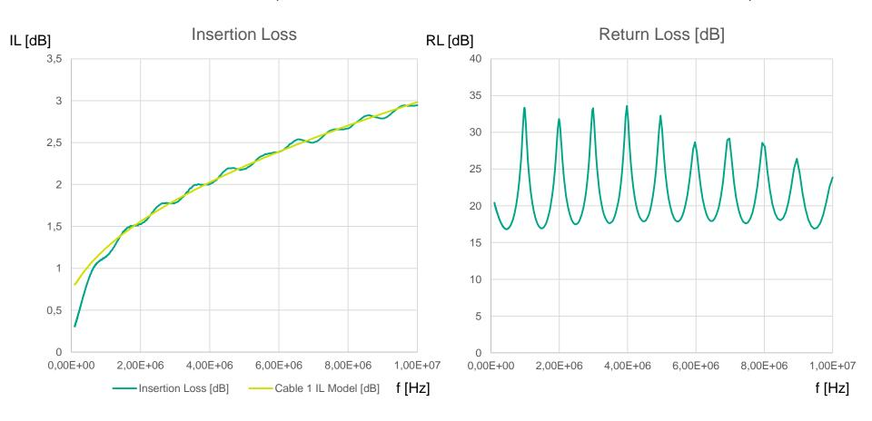
The oscillations are coming from reflections at the cable end due to impedance mismatch with the termination network.
