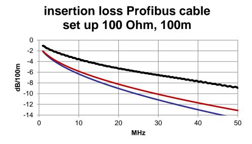
100m measured profibus cable Calculated cable portion Type B 802.3bp upscaled from 40m to 100m Calculated 100 m cat5 cable
