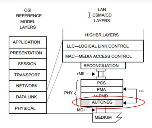
MDI = MEDIUM DEPENDENT INTERFACE MII = MEDIA INDEPENDENT INTERFACE AUTONEG = AUTO-NEGOTIATION PCS = PHYSICAL CODING SUBLAYER PMA = PHYSICAL MEDIUM ATTACHMENT PHY = PHYSICAL LAYER DEVICE PMD = PHYSICAL MEDIUM DEPENDENT
