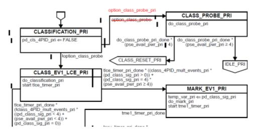
4. change the following state machine for the primary and secondary as shown for the primary.
