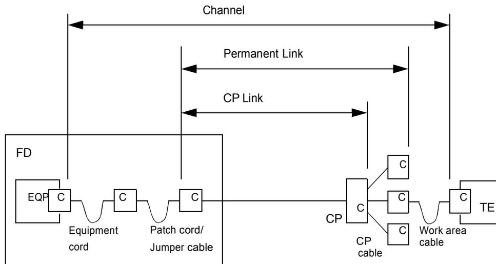
FD = floor distributor; EQP = equipment; C = connection (mated pair);
