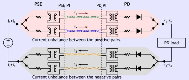
In addition, on the PD side, we need to specify that current specifications apply to the negative pair (given that one or two positive pairs may conduct).
