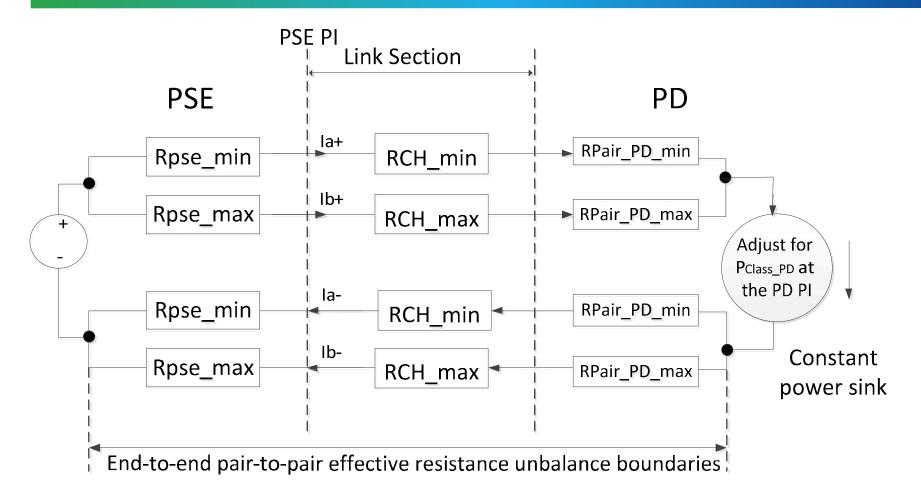
All the unbalance pair-to-pair requirements in D3.0 where derived from this model. The details of the components used in this model are shown in Annex B.
