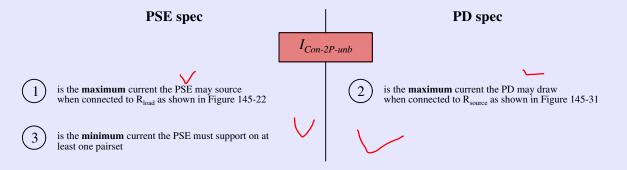
Because the same parameter is used for all 3 requirements, there is no margin between the maximum current that can flow (and must be supported), and the minimum current that a PSE must support. Additionally, because  $I_{Con-2P-unb}$  is defined as a minimum, but used twice as a maximum, we have the potential for confusion.
