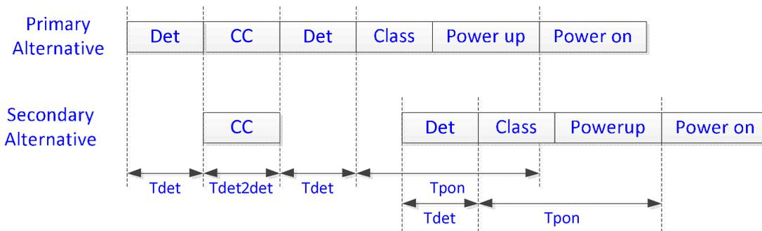
Figure 145B-6A—PSE implementing CC\_DET\_SEQ=1, do\_cxn\_chk result is dual, staggered detection
