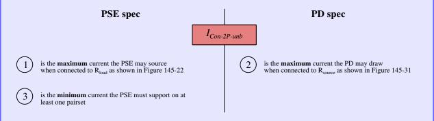
Because the same parameter is used for all 3 requirements, there is no margin between the maximum current that can flow (and must be supported), and the minimum current that a PSE must support. Additionally, because  $I_{Con-2P-unb}$  is defined as a minimum, but used twice as a maximum, we have the potential for confusion.
