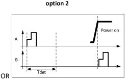
CC\_DET\_SEQ=3 for dual-signature PD is currently used in the state machine by the condition: (!pwr\_app\_sec \* pwr\_app\_pri) which means that we need clarify what is staggered detection for single-signature and dual-signature.
