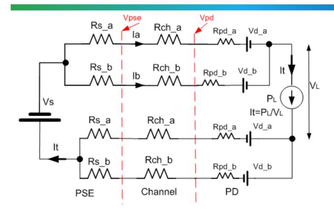
PD diode voltage differences Vd\_a, Vd\_b.
