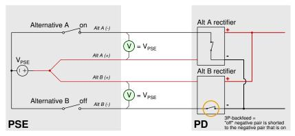
Just like the PSE shorts the positive pairs together, the some PDs short the negative pairs together when exposed to 3-pair power ( $2 \times positive$  and  $1 \times positive$  voltage).
