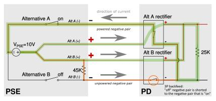
If the PSE ties an "off" negative pair to the positive (via a discharge resistor) and the PD connects the negative pairs together, this causes this resistor to appear in parallel to the PD detection resistor.
